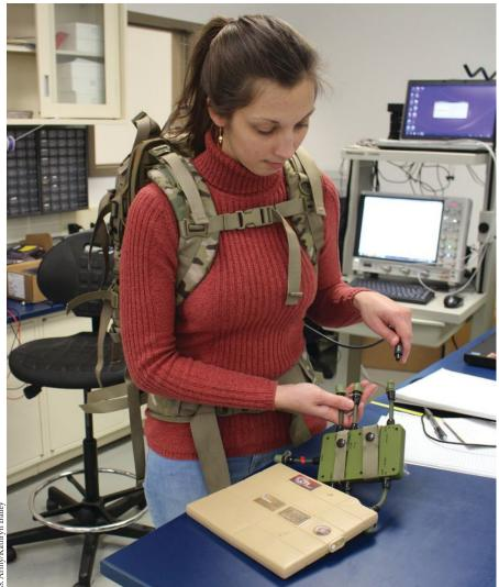
The Integrated Soldier Power and Data System, demonstrated here by an Army engineer, harvests energy to charge a battery that powers soldiers' wearable electronic equipment.
